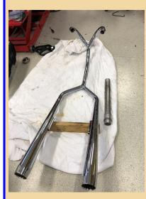
Dr. Blair used computer simulations of the exhaust pressure waves to develop the exhaust system and that is where it was determined the 2 into 1 into 2 pipe system would improve Commando performance. The system used the widely popular Dunstall Decibel silencers that he produced since about 1968. It is said that one year he produced 24,000 Decibel silencers, which have been copied ever since.
