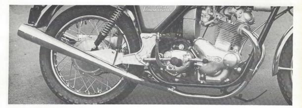
This unique and unusual exhaust system designed in conjunction with Dr. Gordon Blair at Belfast University, offers greatly improved performance due entirely to the efficiency achieved by the design. It consists basically of two small diameter pipes coming from the exhaust ports and joining into one larger pipe which eventually splits back into two to join the Dunstall decibel patent silencers.
