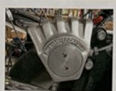
Rear brake is also a disc, and works well enough, especially with entirely new internals
