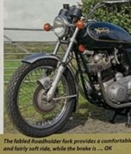
The fabbed Roadholder fork provides a comfortable and fairly soft ride, while the brake is... OK
