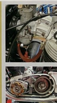
Opinions on the original starter are everywhere and very varied. This one has worked perfectly so far. It drives through a heavily revised primary side.
