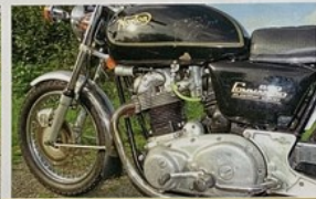
The biggest batch of changes for the MK3 is most visible on the drive side. The left-foot gear shift is an instant recogniser, as is the electric start, which drives the crankshaft via a geartrain. Whereas the earlier Commandos used just a single bolt to secure the outer chaincase, the MK3 uses lots. No idea why.
