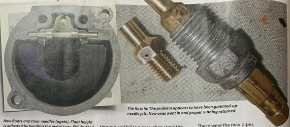
New floats and their needles (again). Float height is adjusted by bending the metal tags. FW decided against this.
