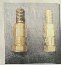
Jets old and new. Upping the jet size made no difference to the engine's running
