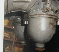
Fitting socket head screws for the float bowls makes access easier than with a screwdriver. Remove the left-side float bowl first
