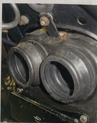
Even the connector hoses were replaced. The first of the new ones is on the right
