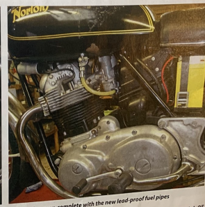
All together now, complete with the new lead-proof fuel pipes
