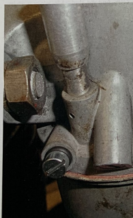
New screws and O-rings: one for each carb
