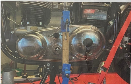
Holding the primary cover on
