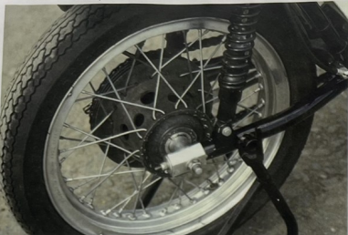
Conical rear hub holds the six drum brake, and the chain adjusters look meaningful too
