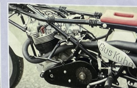
The rider's left foot changes gear, surprisingly, while the cover over the transmission has its own rubber mountings
