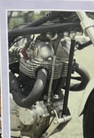
Although there is no actual set of front downtubes, there is a vertical strut to provide positive location of the engine
