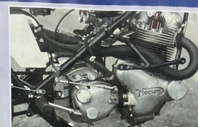
The entire unit is mounted rigidly in the frame and the right-side pedal operates the rear brake
