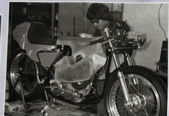
Norton's 1972 factory racer, complete with its pannier fuel tank; lowering the centre of mass is a racer's priority
