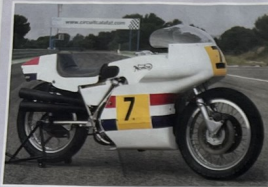
Norton's 1972 factory racer, complete with its pannier fuel tank; lowering the centre of mass is a racer's priority
