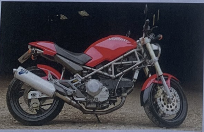
A Ducati Monster, showing how the engine mounts, and the complete absence of front downtubes
