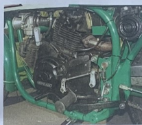
The Ducati engine hangs from a substantial bracket gripped by the top rails. At the rear, its mount is clamped by similarly substantial plates attached to the featherbed's gussets. Note also the substantial brake pedal, and the gearchange crossover
