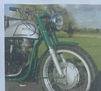
The stock Norton 8-inch s/s drum has been converted to twin leading shoe operation. FW would have preferred twin discs
