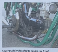
As Mr Builder decided to retain the front downtubes, the right frame rail needed to move a little to accommodate the engine's wet sump
