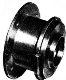
On the left you see the drive-side main-bearing housing Lacey fits to Manx Norton crankcases as a matter of routine. The bearing carries a 4in-diameter flange and is retained externally by a locking ring
