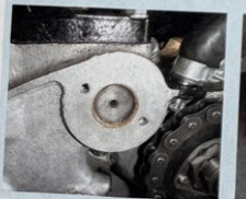
The camshaft tunnel leaked, so Paul employed a coin to seal it. Thanks, your majesty!
