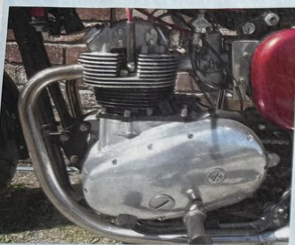
Norton's prototype unit twin: neat and compact, and with the camshaft behind the cylinders, unlike their earlier engines
