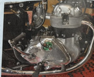
The timing side, showing the Pazon ignition system and a little Norton ancestry in the rocker box layout
