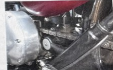
Drive chain run and angle were the source of much disturbing noise...
