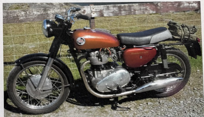
Drive chain run and angle were the source of much disturbing noise...
