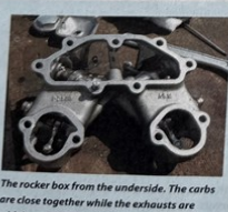
The rocker box from the underside. The carbs are close together while the exhausts are widely splayed, aiming for a straight path for the combustion gases
