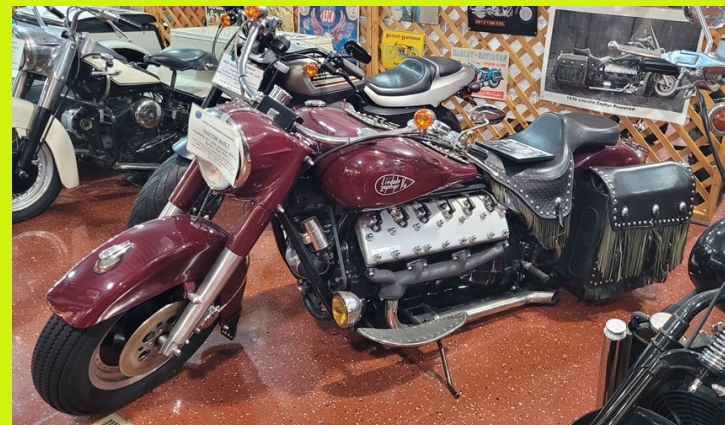
WORLD OF MOTORCYCLES MUSEUM, INC. CUSTOM BUILT POWERED BY: 1939 LINCOLN ENGINE Builder: Duke Olson This motorcycle was custom built and is powered with a 1939 Lincoln Zephyr car engine. Water cooled, flat head V-12, with 1-speed transmission and stock automotive clutch.
