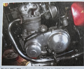
Norton Atlas 750 engine mates neatly with the AMC alloy primary chaincase. It's a better case than the pressed steel contraption used on earlier Norton twins
