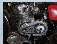
Primary cover removal required the removal of the left exhaust pipe and footrest
