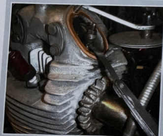
Checking the valve clearances
