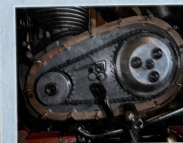
New paper primary cover gasket was a goat's too small
