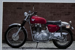
In broad terms, the Norton P11 series combines the Norton Atlas engine with the bicycle frame from the Matchless G8SCS scrambler. There are many detail differences, one being the adoption for the Norton of a road-type rear hub, rather than the Matchless G8SCS wheel from the G8SCS. This is such a Matchless, boasting the same AMC Teledraulic fork and AMC brake as the Norton
