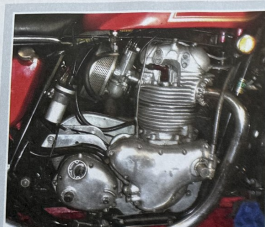
Slightly inclined engine leans forwards less than its Commando counterpart, but shares the silver barrels of the early models
