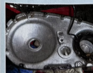
Alternator stator lives in the primary cover. Note the alloy welded repairs
